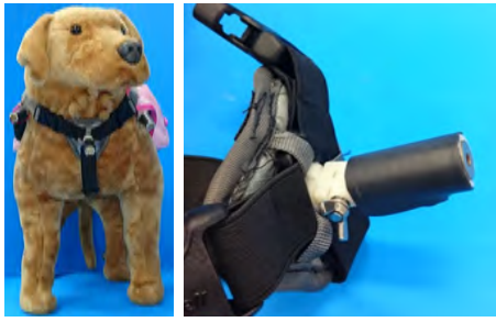
Fig. 9. Canine suit equipped with three lasers: (left) Front view of the suit, (Right) Laser device that consists of a laser and a 2 axes laser holder.
